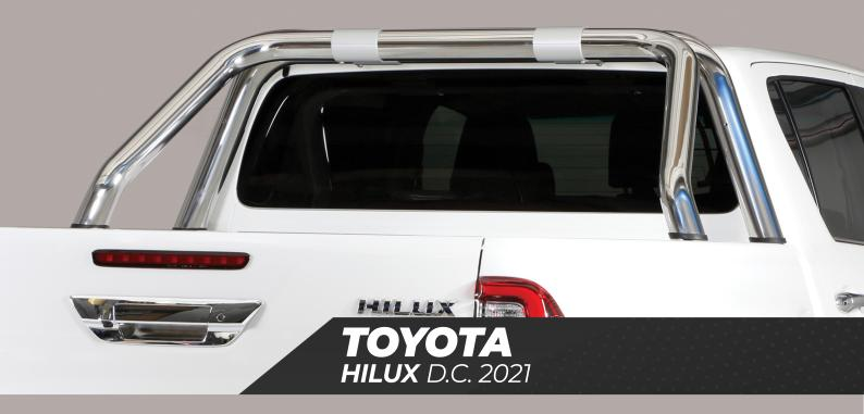
**RLD/K/410/IX** Roll Bar Mark design Ø 76mm
